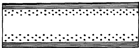
paste fired onto steel, part of the element diffuses in
